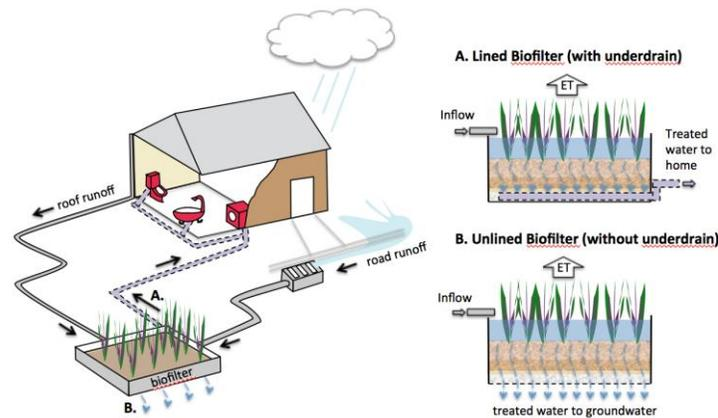
*Biofilters are low-energy distributed treatment technologies that capture and treat stormwater (from roofs and roads) using biological and physicochemical processes.*
