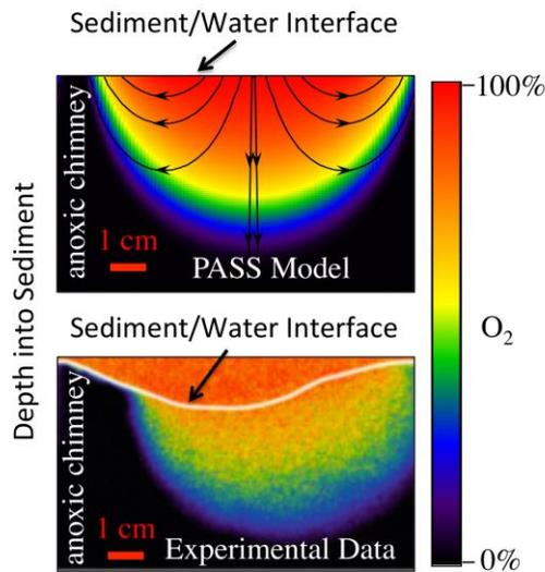
*Process-based models are being developed to quantify the biogeochemical removal of nutrients in the hyporheic zone of natural and engineered streams.*
