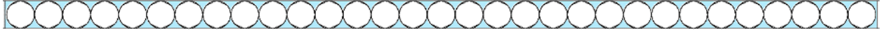
Figure 7: Sideview of a compound refractive lens diagram with polystyrene spheres (outlined in black) within a liquid refractive material (shaded in blue)
