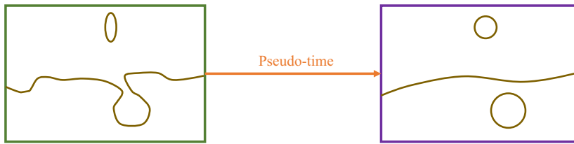
Figure 7. Sketch of how a pseudo-surface tension could create low DoF representations of a complex two-phase interface.
