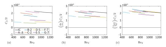
FIG. 8. (a) Skin friction coefficients without transformation, (b) integral transformation based on stressweighted density, and (c) integral transformation based on the ratio of the compressible and incompressible AMI length scales.
