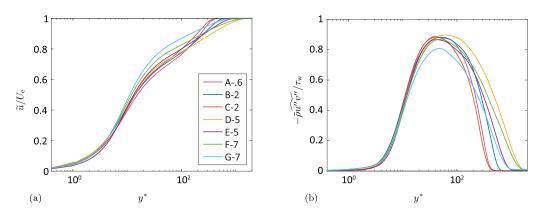
FIG. 2. Normalized Favre averaged (a) velocity by the edge velocity and (b) Reynolds shear stress by the wall shear stress. The profiles are plotted at  $Re_2$  shown with \* in Fig. 6(a).
