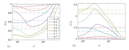
FIG. 4. Normalized (a) average density by the edge density and (b) Favre average viscosity by the edge viscosity. The dashed lines in (a) show  $\rho_2$ , Eq. (16). Also, the dashed and dotted lines in (b) represent the value of  $\mu_2$ , Eq. (11), and  $\mu_H$ , Eq. (28), respectively. The profiles are plotted at Re<sub>2</sub> shown by \* in Fig. 6(a), except for  $\mu_H$  that is plotted at Pe<sub>H</sub> shown by \* in Fig. 10(a).
