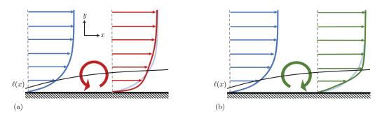
FIG. 1. Schematic of applying torque with respect to axis  $\ell(x)$  (black solid line) to the blue velocity profile: (a) applying a counterclockwise torque and (b) applying a clock wise torque.
