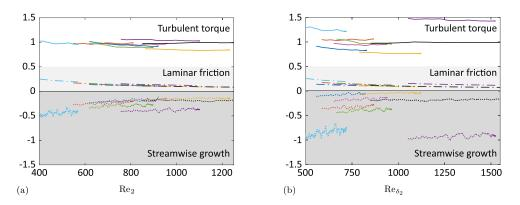
FIG. 7. Normalized contribution of *turbulent torque* (white background), *laminar* friction (light gray background), and *streamwise growth* (dark gray background) by  $C_f/2$ : when the reference viscosity (a)  $\mu_{ref} = \mu_2$ , and (b)  $\mu_{ref} = \mu_w$ . In (b),  $\text{Re}_{\delta_2} = U_e \rho_e \delta_2 / \mu_w$  is the Reynolds number based on the wall viscosity.
