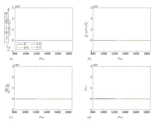
FIG. 13. Contribution of (a) deviation from reference viscous transport, (b) flux due to the edge pressure gradient, (c) nonisothermal wall temperature, and (d) the negligible terms due to departure from the BL approximations to the MTEI equation, Eq. (23), based on  $\mu_{ref} = \mu_H$  and  $\ell = \ell_{H,C}$ .
