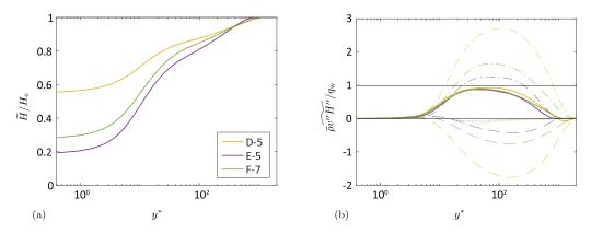
FIG. 3. Normalized Favre averaged (a) total enthalpy by the edge total enthalpy, and (b) wall-normal velocity and total enthalpy turbulent covariance by the wall heat flux (for study cases of MTEI equation). In (b) the dashed, dashed-dotted, and dotted lines represent  $c_p \overline{\rho} \widetilde{T''v''}$ ,  $\overline{\rho} \widetilde{uu''v''}$ , and  $\frac{1}{2} \overline{\rho} \widetilde{u''u''v''}$ , respectively. The profiles are plotted at Pe<sub>H</sub> shown with "\*" in Fig. 10(a).
